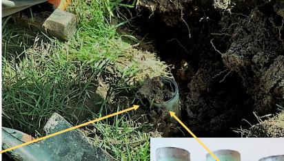
Pipe takes a soil plug for leaching test – In the lab 100ml of clean rainwater is poured on top to monitor how long it takes to permeate the soil and how much is absorbed.
